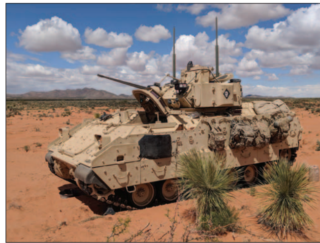
Above: The Fort Bliss training area is full of features like training villages that are used in urban warfare scenarios. Left: A Bradley Fighting Vehicle is designed to carry infantry or cavalry scouts and is considered one of the Army's most versatile platforms.
