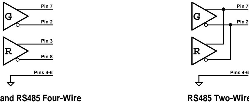
Figure 5 – P1/P2: Selectable Serial Interface Pin Assignment - RS422/485 Configuration
