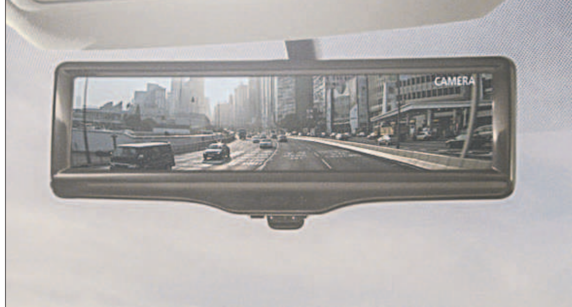
THIS NISSAN Smart Rearview Mirror provides a split screen view with side cameras to see what's on either side as well as what is behind the vehicle. More than two-thirds of the most popular vehicles have back up cameras available.
