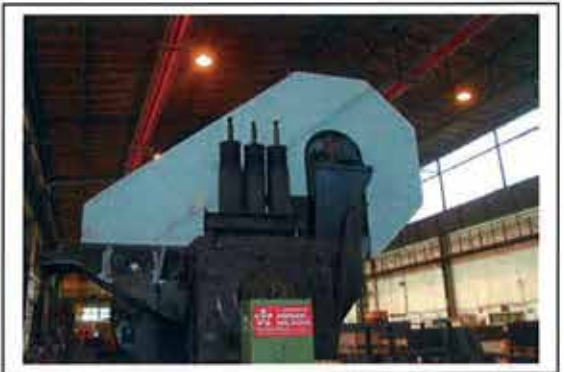
Figure 4.8b: Simple cover for dangerous parts,
