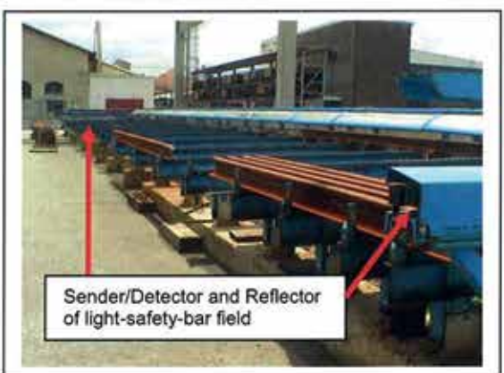
Figure 4.9b: .....and in horizontal position additionally for surveillance that nobody is staying within an area – see example automatic conveyor area of sawing-drilling unit. There are different classes of light/lasers (different range in covered distance and number of rays per meter (for different stages of safety like "finger-proof", "arm-proof" or "body-proof")); outdoor and especially above 30m distance light bars will be problematic due to false signals (rain/fog/birds...)
