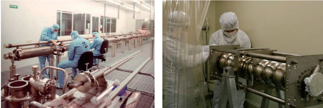
FIGURE 1.2-4. Clean room environments are mandatory. Left: the assembly of eight nine-cell TESLA cavities into a cryomodule string at DESY. Right: an ICHIRO nine-cell cavity is prepared for initial tests at the Superconducting RF Test Facility (STF) at KEK.
