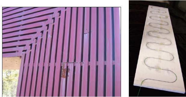
Figure 3.9: A view of one of the ND280 magnet yokes with air gaps visible (left) and an SMRD ‘slab’ (right) [18].
