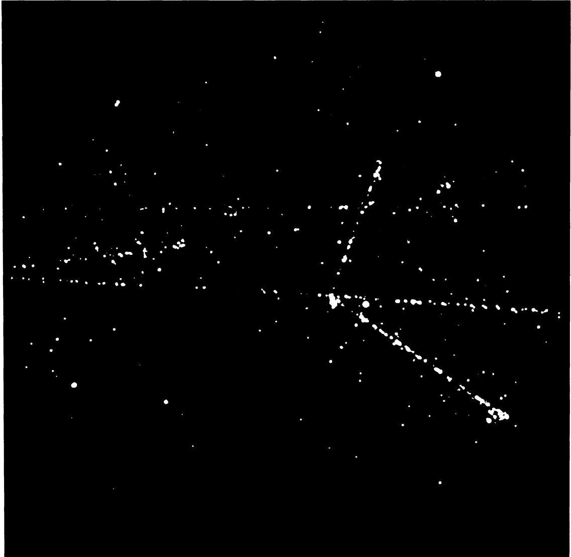
Figure 24—Example of a 5 GeV/c \pi^- interaction in the CERN-RAL-MPI (Munich) 'scintillation chamber'. The longest track length is 18 mm and the typical spot diameters are 80 \mu\text{m} . The track residuals are \sigma \sim 20 \mu\text{m} .
