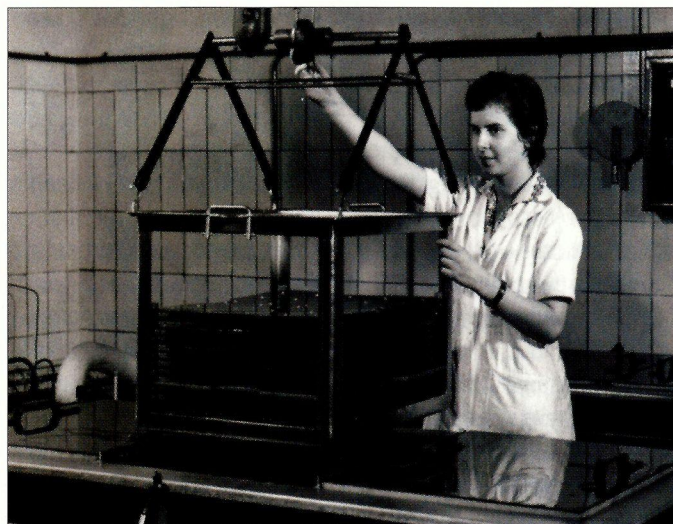
In the 1950s photographic emulsion was, beside the cloud chamber, the dominant method for the detection of highly energetic cosmic-ray particles. Following a 1955 initiative of Cecil Powell, a developing bath for emulsions was installed in the Zeuthen laboratory.
