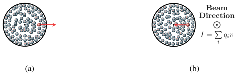
Fig. 2: (a) Charges: repulsion. (b) Parallel currents: attraction
