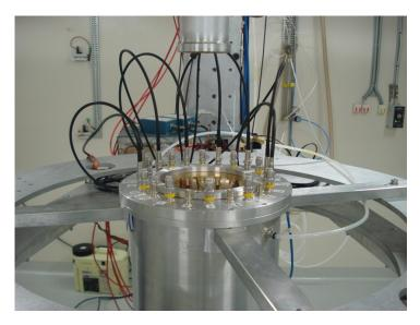
**Fig. 1:** A view of the chamber housing the samples and detectors, and the associated electronics placed in the neutron beam in EAR-2. The neutron beam arrives vertically from below and then continues in the value tube above the chamber and onto the beam dump a few meters later. Approximately 15-20 cm of air are present before and after the chamber.
