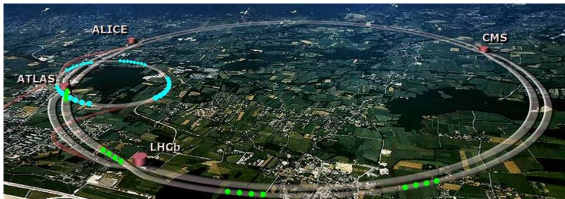
Figure 1.8: Lying deep under ground (122m to lowest point), the LHC has a 27 kilometers circumference. It lies between the Jura mountains and the Alps, covering both French and Swiss soil.
