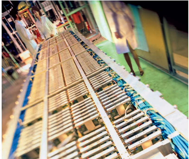
45. View of one of 18 TOF supermodules during construction (photo: Antonio Saba).
