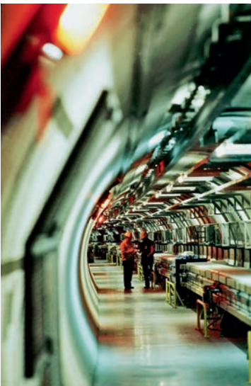
7. The Large Electron-Positron collider. LEP ran from 1989 to 2000. The maximum energy achieved was 104.5 GeV per beam. At that energy, it was losing more than 5 GeV per turn due to synchrotron radiation. It was dismantled in 2001 to make way for the LHC.
