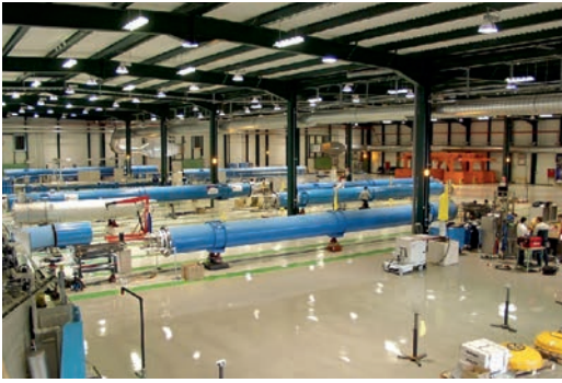
50. Assembly of LHC magnets in their cryostats.
