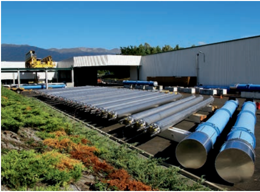
6. Delivered cold masses awaiting cryostating and testing (September 2003).
