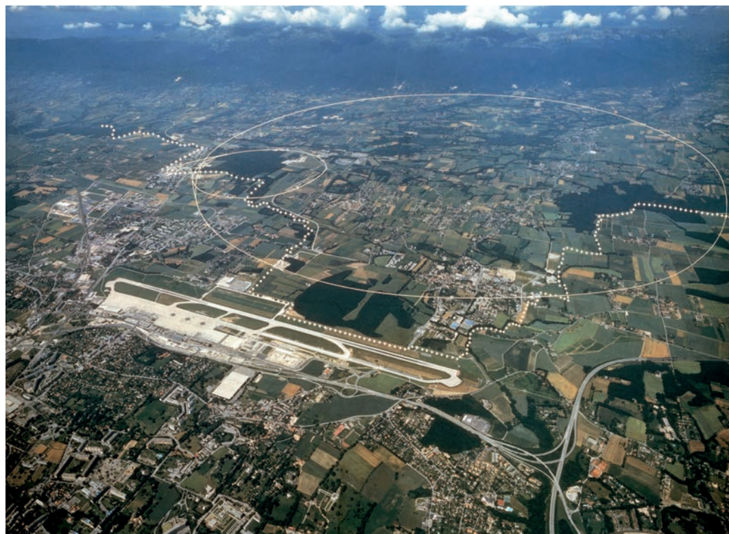
3. An outline of the position of the 27-km LHC ring. The airport of Geneva can be seen in the foreground. The dotted line is the border between Switzerland and France. The LHC tunnel is approximately 100 meters underground; nothing can be seen from the surface.
