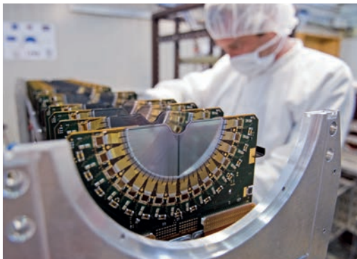
58. (a) A photograph of the assembly of the last module of the VELO system; and (b) a view of the same during installation into LHCb.
