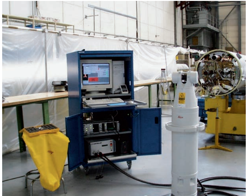
15. The laser tracker developed at CERN to measure the magnet shape, with its accompanying instrumentation.
