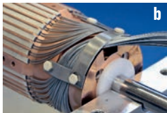
6. Two views of the 13-kA high-temperature superconducting leads used in the LHC: full lead (a) and detail (b) showing a close-up of the lower part. In (b), the transition between the high-temperature superconductor (on the left) with the low-temperature superconductor (on the right) is visible. Resting in liquid helium, the low-temperature superconductor is connected to the busbars conveying the current to the LHC magnets. (courtesy of A. Ballarino, CERN).
