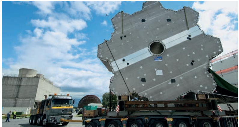
2. ATLAS toroid magnet end cap being transported to ATLAS Point 1.
