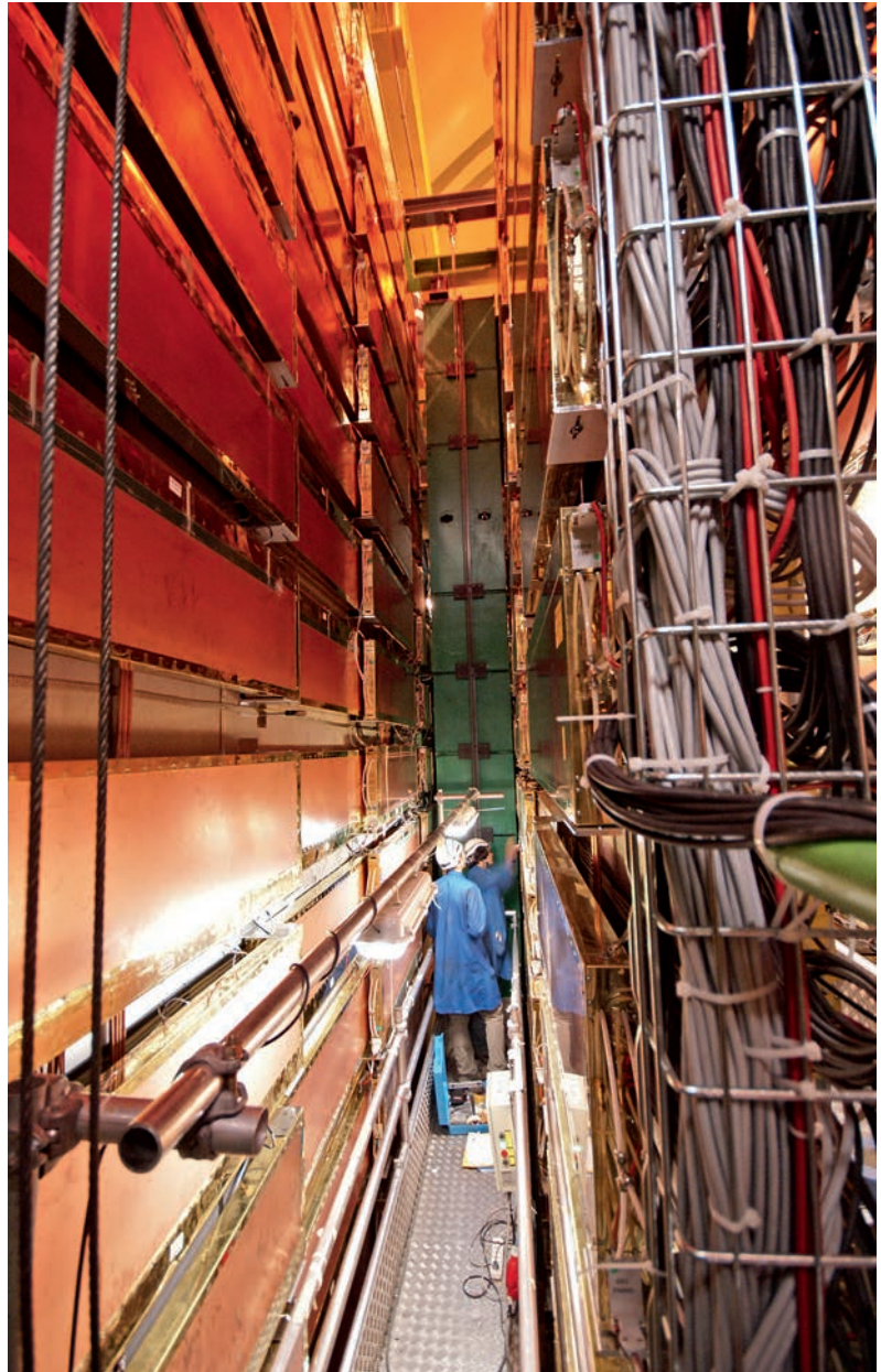
63. An inside view of the LHCb muon detection system, showing two stations on either side and a green iron absorber block in the back.
