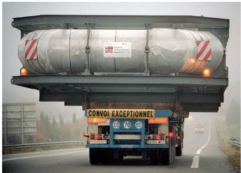
15. Transport of the ATLAS barrel toroid to CERN.
