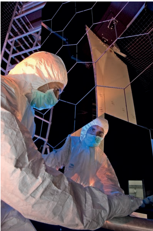
59. The installation of the high-precision spherical mirrors for the RICH detector. These mirrors will focus Cherenkov light, created by the charged particles that traverse this detector, onto the photon detectors.
