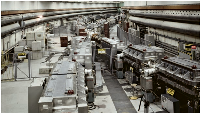
6. The Intersecting Storage Rings was the first proton-proton collider. The two separate rings can clearly be seen. In the ISR, accelerator physicists learned how to store proton beams and experimentalists learned how to build detectors.
