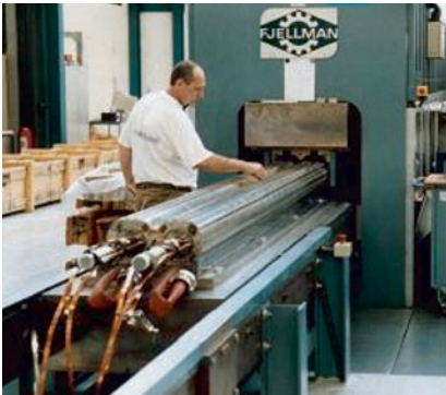
16. LHC coils ready for the collaring (left) and cold mass ready for welding (right).
