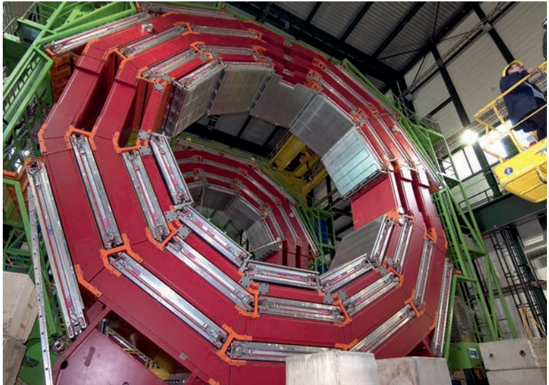
8. Installation of the barrel muon detector of the CMS showing how the muon system is structured with alternating layers of iron return yoke (red) and muon detection chambers.
