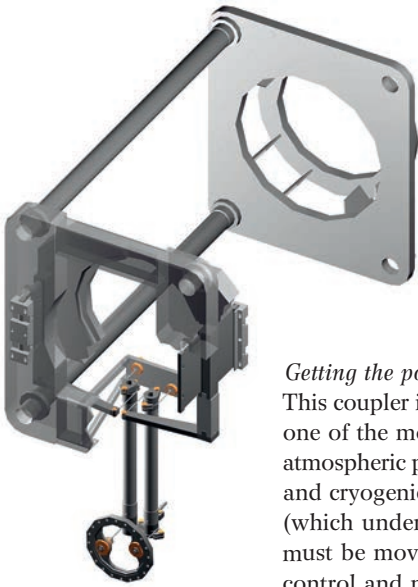
93. The cavity is held at its ends by the two square plates. A system of lever arms allows the two “blades” to be bent, compressing or stretching the cavity.
