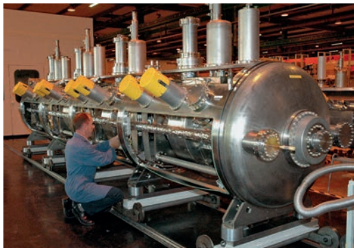
91. Final touches to a superconducting RF module after assembly in the clean-room (in the background).
