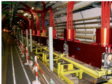
77. The 15 extraction kicker magnets for the beam 1 dump, installed in the LHC tunnel.
