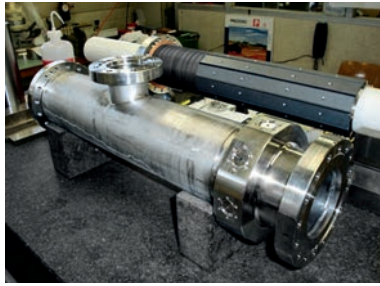
101. The longitudinal pick-up with, left, the center cylinder (beam-tube) removed to show the ferrites and, right, the completed pick-up with four of the eight connectors visible on the left-hand end and the pumping port in the middle.
