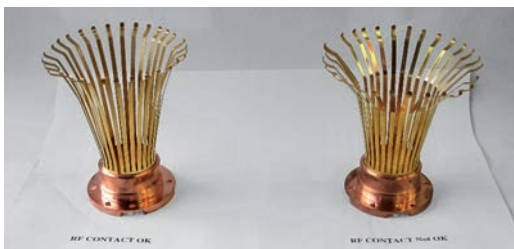
42. Sample contact fingers showing the critical parameters as specified and “as-built” for the PIMs.
