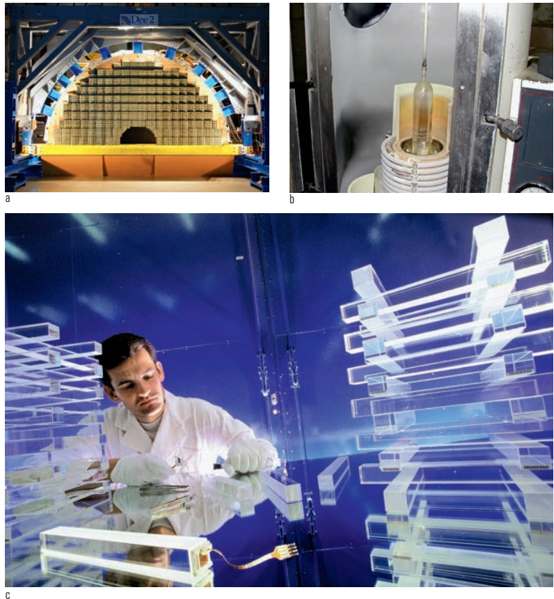
20. Some views of the lead-tungstate-crystal technology used for the electromagnetic calorimeter: (a) a view of one of four “Dees” with around 3,700 endcap crystals mounted on a backplate; (b) a lead tungstate crystal ingot at the end of a 3-day growing cycle; and (c) lead tungstate crystals under inspection at CERN (photo: Peter Ginter).
