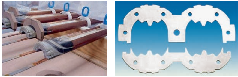
14. LHC coils ready for assembly (left) and collars (right).
