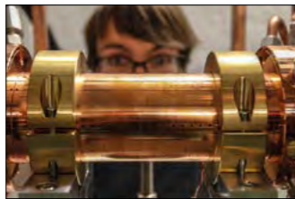
CLIC tech Prototype of the CLICX-band structure at the heart of the CompactLight linac.
