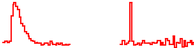
Figure 66b: The deconvolution of the signal of a silicon detector. The amplifier has a time constant of 50ns.
