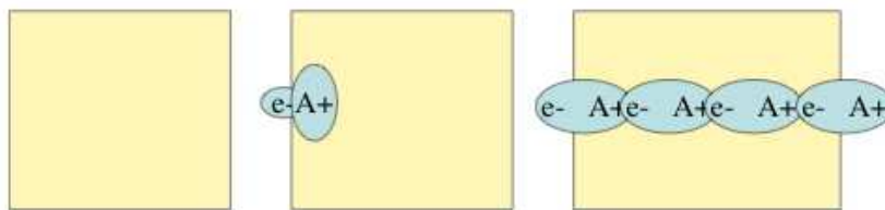
Fig. 16: Charge transfer in a dielectric medium, via a sequence of local polarizations
