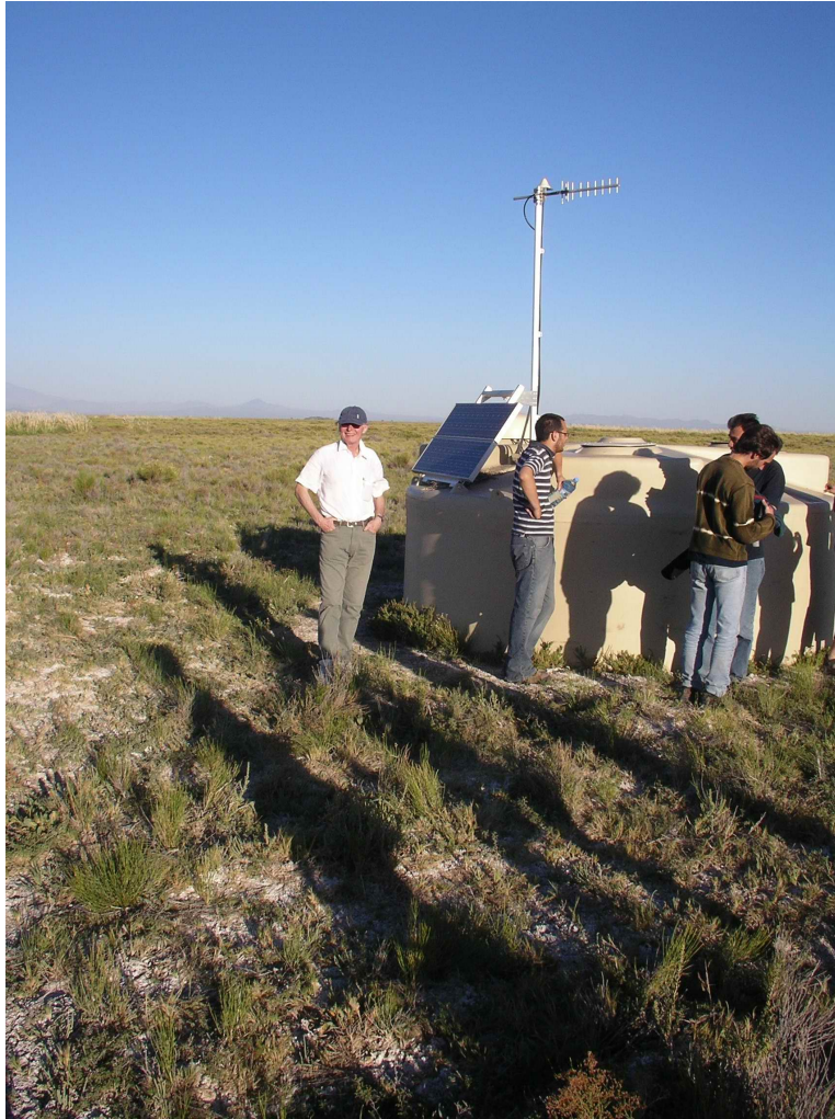
Fig. 22: Photograph of a surface detector unit
