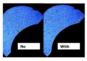
A hemispheric protrusion on an airframe at near sonic flight conditions suffers a tremendous degree of flow separation behind the unsteady shock that forms near its apex. Such condition can be alleviated by applying active flow control (AFC). However, due to the performance degradation occurring with standard AFC devices at high flight velocities combined with impractical weight requirements, a new system that was developed at the
