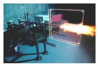
A pulse detonation engine (PDE) offers few moving parts, high efficiency, high thrust, low weight, low cost, and ease of scaling. These make the PDE an attractive alternative to jet turbine engines for small disposable engines. The near constant volume heat addition process, along with the lack of a compression cycle, lend to the high efficiency and specific impulse, simplicity, and low-cost of pulse detonation engines.
