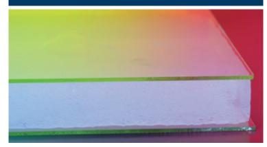
For example, the ISOGEL® grade of silica aerogel in granular form can be incorporated into mortar used for façades in order to give a building a mineral skin with insulating properties that are significantly greater than other insulating materials of a similar thickness.
