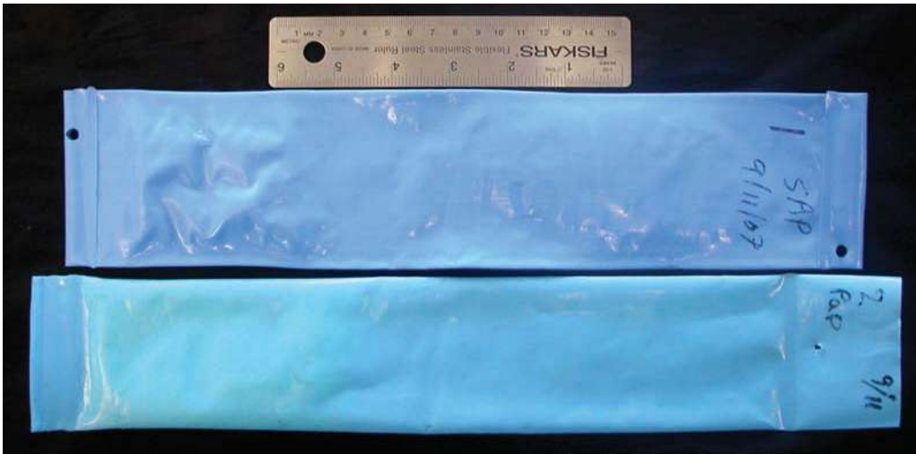
Figure 26.2— Commercially available polyethylene sleeves used to enclose host monoterpenes (e.g., \alpha -pinene). Synergy Semiochemicals, Corp. (Burnaby, BC, Canada) ultra-high release \alpha -pinene (upper); Contech/Phero Tech, Inc. (Victoria, BC, Canada) ultra-high release \alpha -pinene (lower). Scale from 0 to 6 is inches. (photograph by B. Strom)
