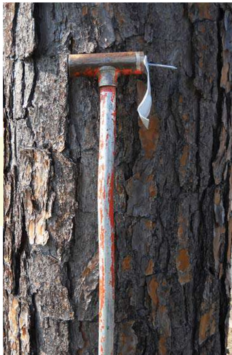
Figure 26.7 —The Hundle hammer (left), and pouch placement on treated trees (right). (photographs by S. Clarke)
