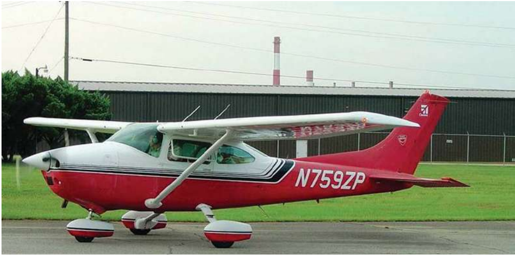
Figure 17.6 —Small, high-winged aircraft, such as this Cessna 182, are typically used for conducting aerial detection flights for SPB infestations. (photograph by Ron Billings, Texas Forest Service)
