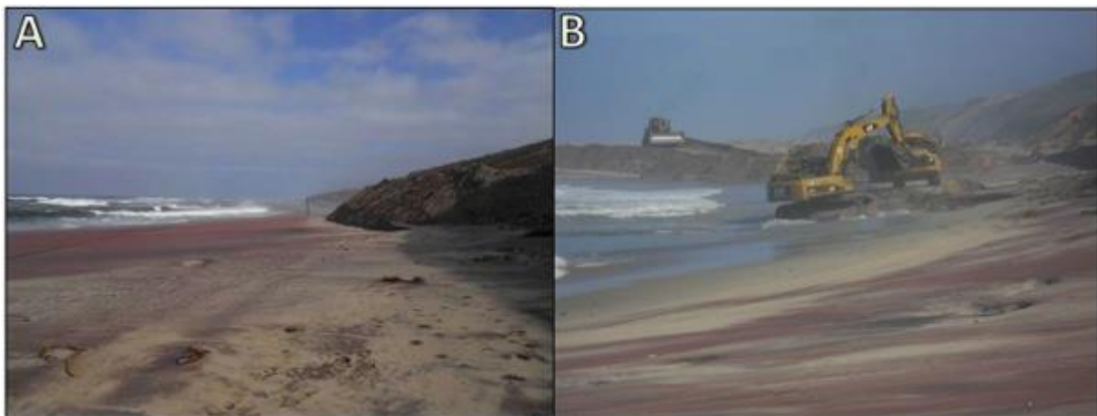
Figure 6.1: MSR mining activities. A: Minerals within the sands of the beach are obvious. B: The mining activity takes place within a very small footprint at any one time and is restricted to the zone between the low tide mark and the 10m buffer zone from the dune vegetation.
