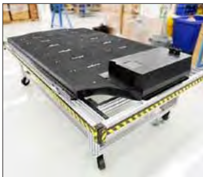
A new flat battery pack will allow Tesla's upcoming Model S luxury sedan to run up to 300 miles on a charge.
