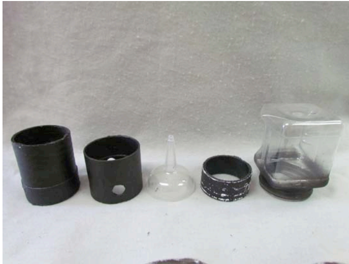
Figure 1. Components used to make improved collar traps. Bait jar, 3-inch PVC collar with \frac{3}{4} inch holes, plastic champagne glass, 3-inch drainage pipe used to connect 32 ounce pinch grip plastic container.
