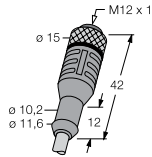
Connector socket M12x1 straight, 5-pin
