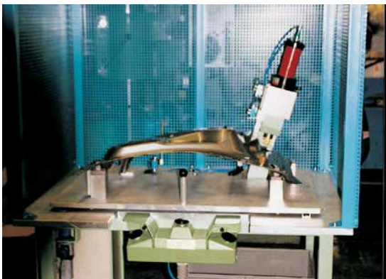
Device for holes Ø 8 in sheet metal
