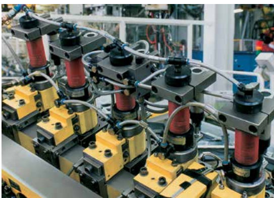
Stamping units placed in line
