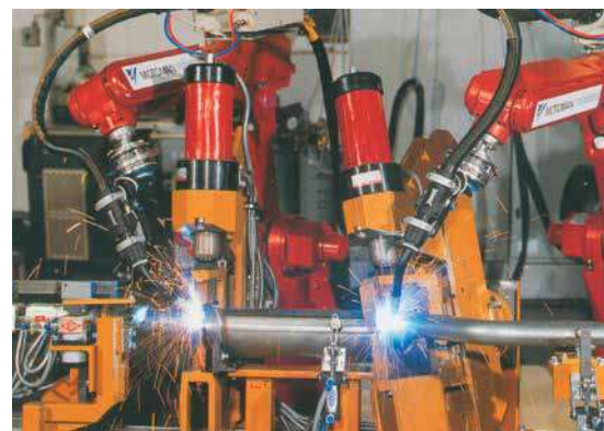
Welding fixture for exhaust components
