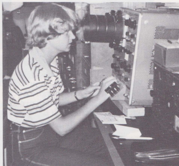
Testing transistor gain and breakdown with the transistor curve tracer.
