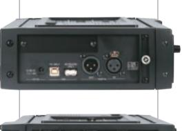
INTERFACING The FR-2 is very well connected: the two analog inputs switchable between Mic & line on XI R connections link to top quality microphone pre-amps with selectable phantom power, while analog out is offered on RCA connectors. Digital I/O is selectable between AES/EBU and S/P-DIF, again on balanced XLR The USB ports allow direct connection to PC and MAC with an additional port allowing for an external keyboard to be used to aid file naming and operation
