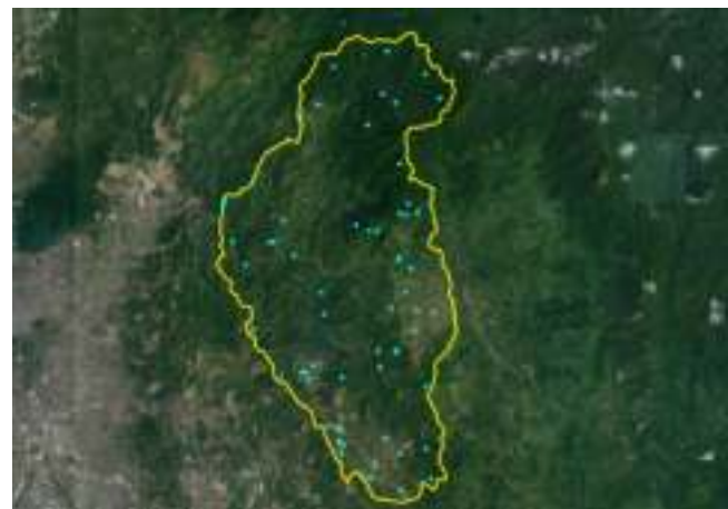
Figure 9. Ground truth points to the accuracy assessment of the classified satellite image
