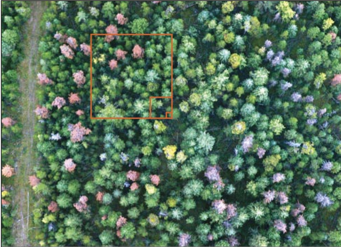
Figure 1. Illustration of information content of three common image spatial resolutions of 30 x 30 m, 4 x 4 m, and 1 x 1 m. Larger pixels tend to amalgamate a greater variety of stand elements.
