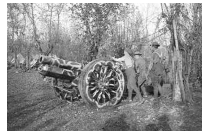
6.2 A 6" 26 cwt howitzer being positioned by troops of the 293rd Siege Battery, RGA - Italian Front © IWM
