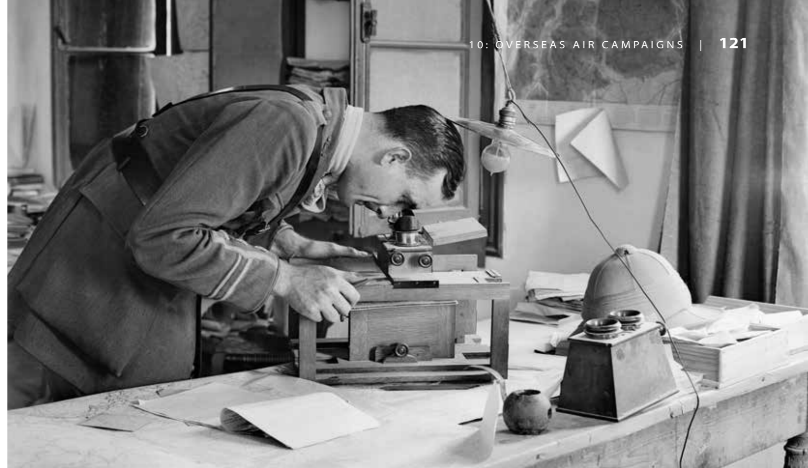
10.12 British Intelligence Officer uses a stereoscopic viewer to interpret aerial reconnaissance photographs on the Italian Front © IWM
