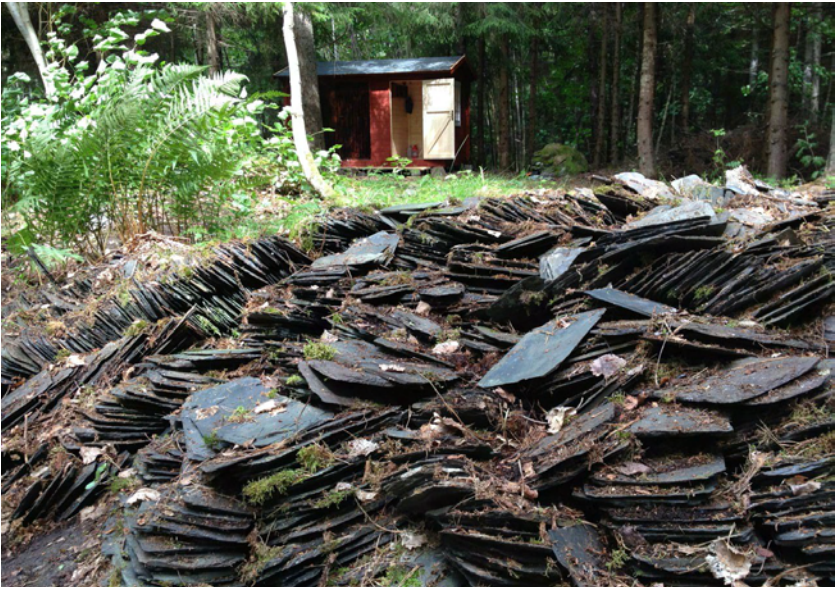
Huge pile of saved hand-cut old 1800s slate shingles from the house roofs, ready to be used again for restored houses. New shed erected 2014 in the background on site of previous collapsed fishing shed. Photo by Anders Rhodin.
