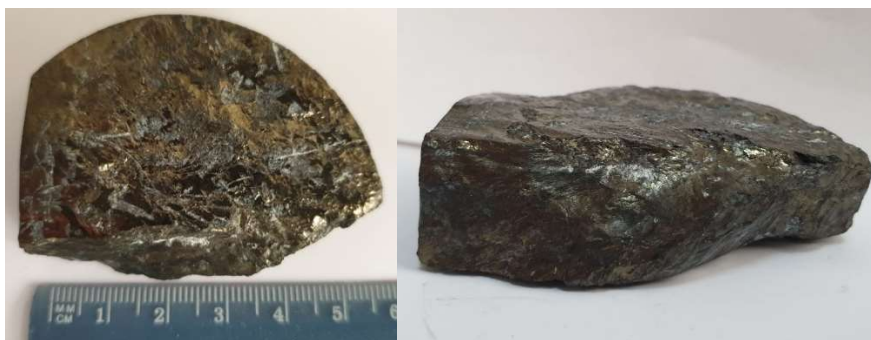
Figure 1. Photos of a typical rock slab (left: upper view of valleriite and accompanying minerals, right: side view showing the thickness of the upper valleriite-bearing layer).
