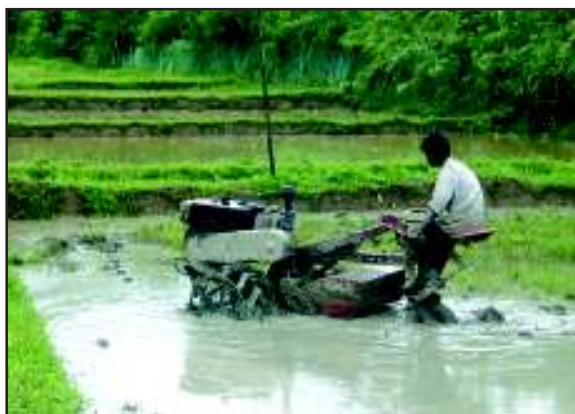
Plate 26, Puddling with power rotary tiller
