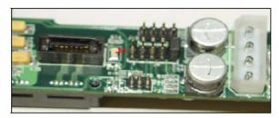
Figure 6 - Installing shunt.
