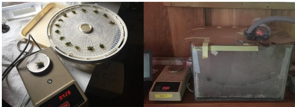
FIGURE 4. (Left) Food dehydrator used in the process of determining desiccation rates of moss samples. Dehydrator was set to a heat of 35°C during sampling. (Right) Glass aquarium and misting apparatus used in the process of determining water capture rates of moss samples. Aquarium was covered and lightly sealed with humidifier entering through the center. Humidifier was set to output 1.04 ml/min for the duration of sampling. Wire mesh elevated samples off the bottom to reduce the effects of pooling water. Samples were placed equidistant from the tube to avoid effects of proximity.
