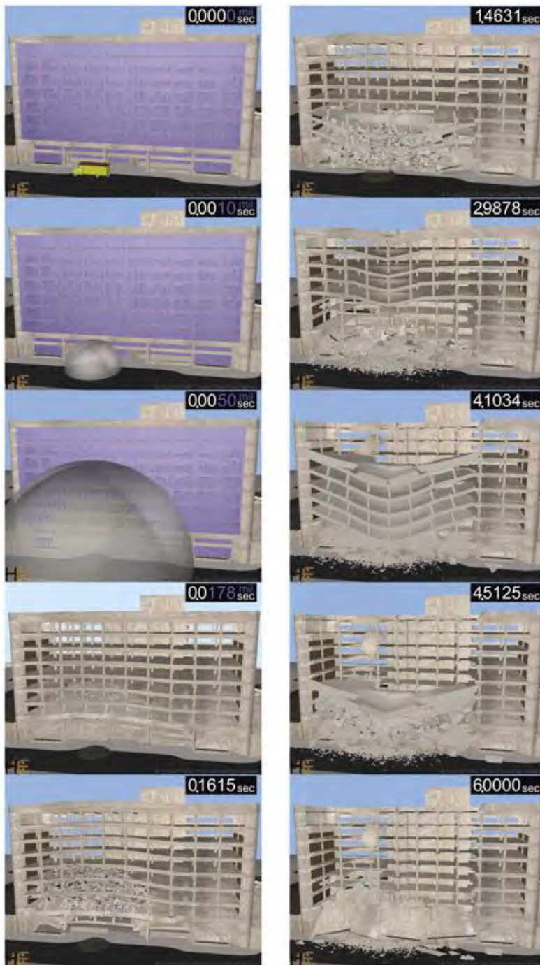
Figure 7: Computer simulation of a blast sequence. Image courtesy of Hinman Consulting Engineers, 2005
