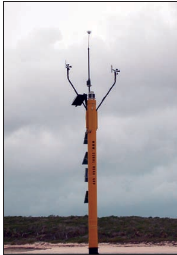
Fig. 1- Installation of the newly designed CREWS monitoring station near the Perry Institute for Marine Science on Lee Stocking Island,
