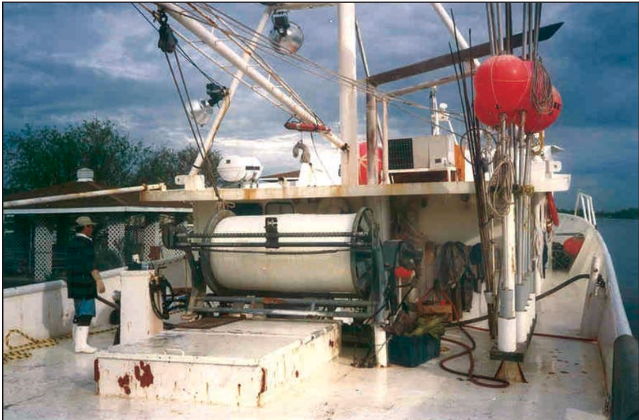
Fig.1: Typical U.S. pelagic longline vessel showing the mainline spool (center), hi-fliers attached at regular intervals along the mainline (right side of picture), and the vessel work deck.
