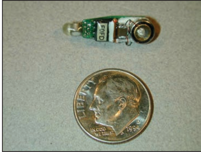
Figure 1. Sample micro-acoustic tag (PNNL Labs) to be used in tracking the movements of juvenile snappers. Photo: T. Carleson, Ph.D.
