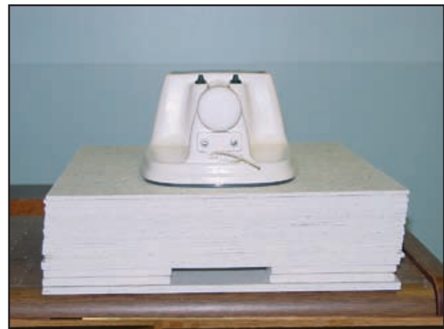
Figure 2. Experimental layout. PIT tag scanner on vinyl tiles with embedded PIT tag.
