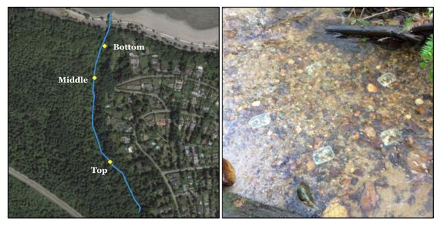
**Figure** 7: Fifteen sediment accumulators were installed in Spanish Bank Creek. The sediment accumulators were installed in Spanish Bank Creek at locations denoted as top, middle, and bottom (left; QGIS Development Team, 2009). Five accumulators were installed at each of the locations, for a total of 15 accumulators (right; Reynolds, 2016).
