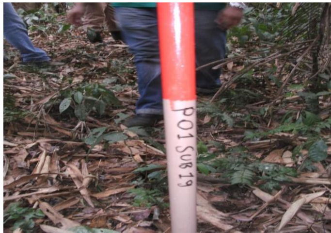
Figure 22 Use of PVC pipe with the top edge end painted in red to sign permanent parcels and the sub-parcels
