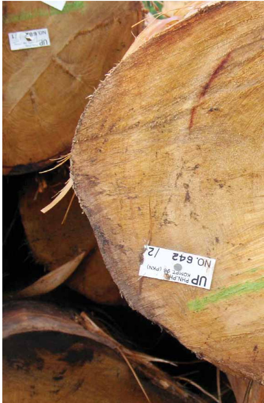
Figure 4.1 Sapwood and heartwood of a G. bancanus log is not distinctly differentiated.
