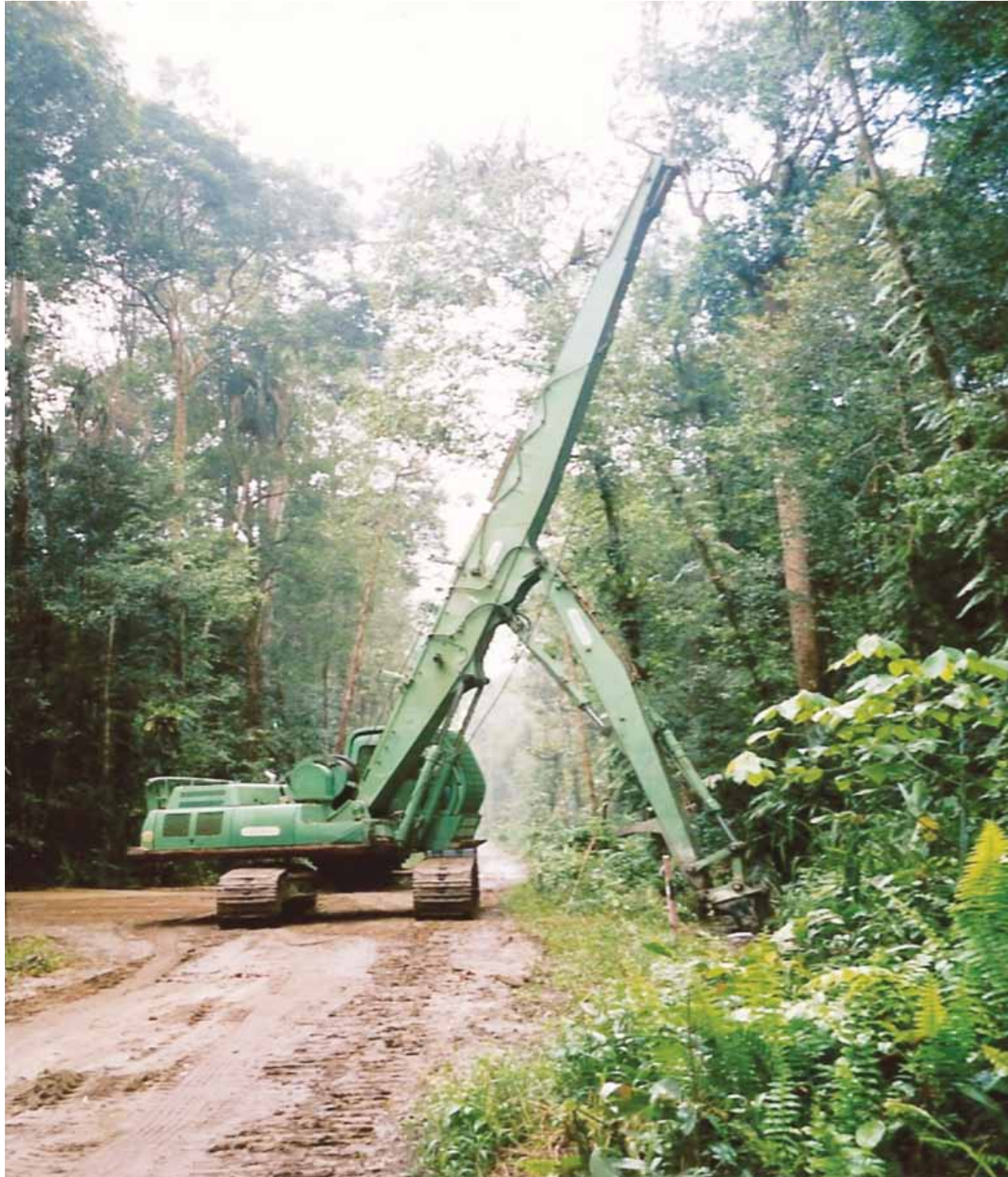
Figure 3.3 The Rimbaka timber harvester minimizes its movement by pulling logs using long cable to reduce damage to the forest floor.
