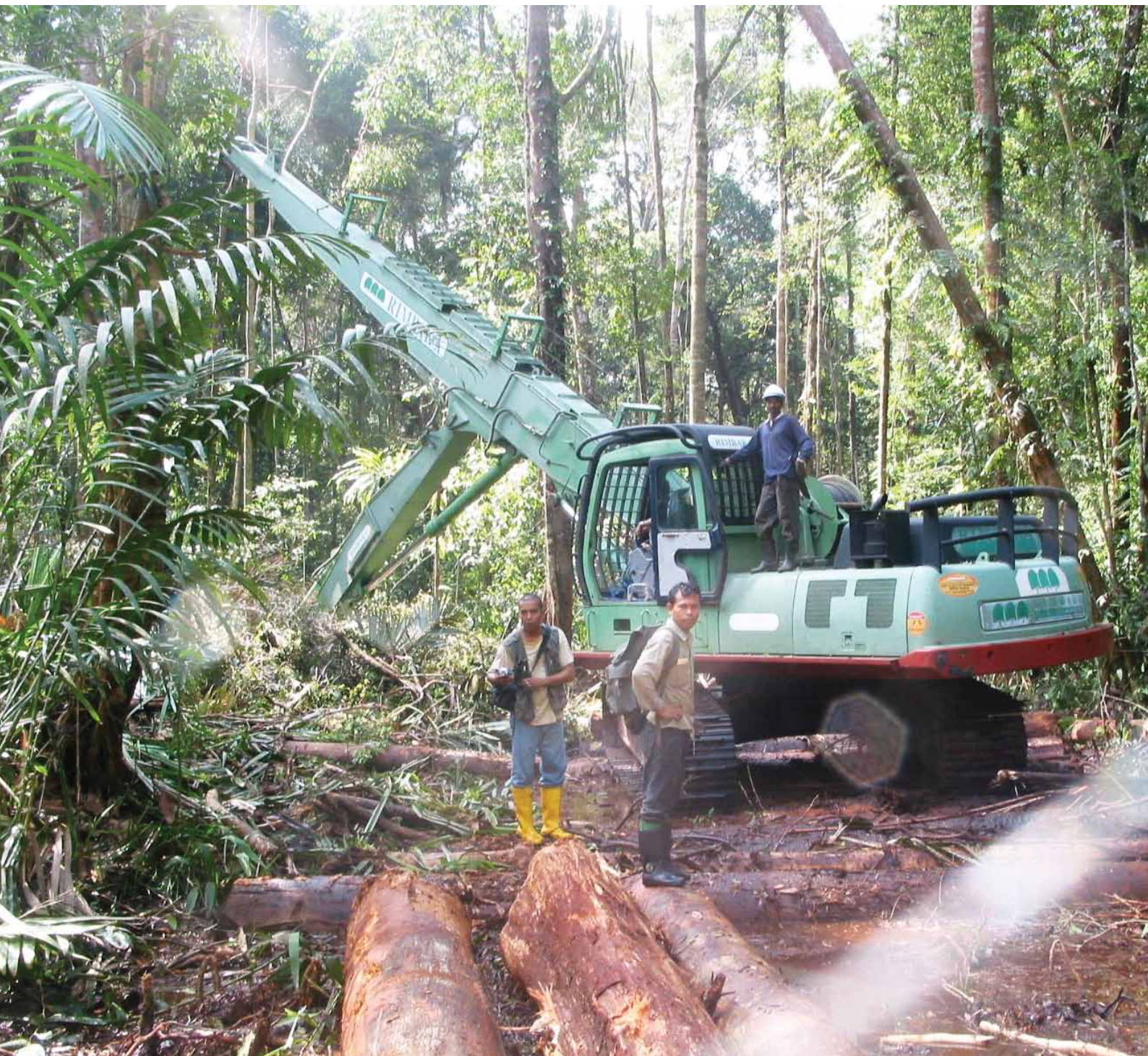
Figure 3.2 Rimbaka timber harvester in action. The use of Rimbaka timber harvester to extract logs in Pekan FR contributes to RIL.
