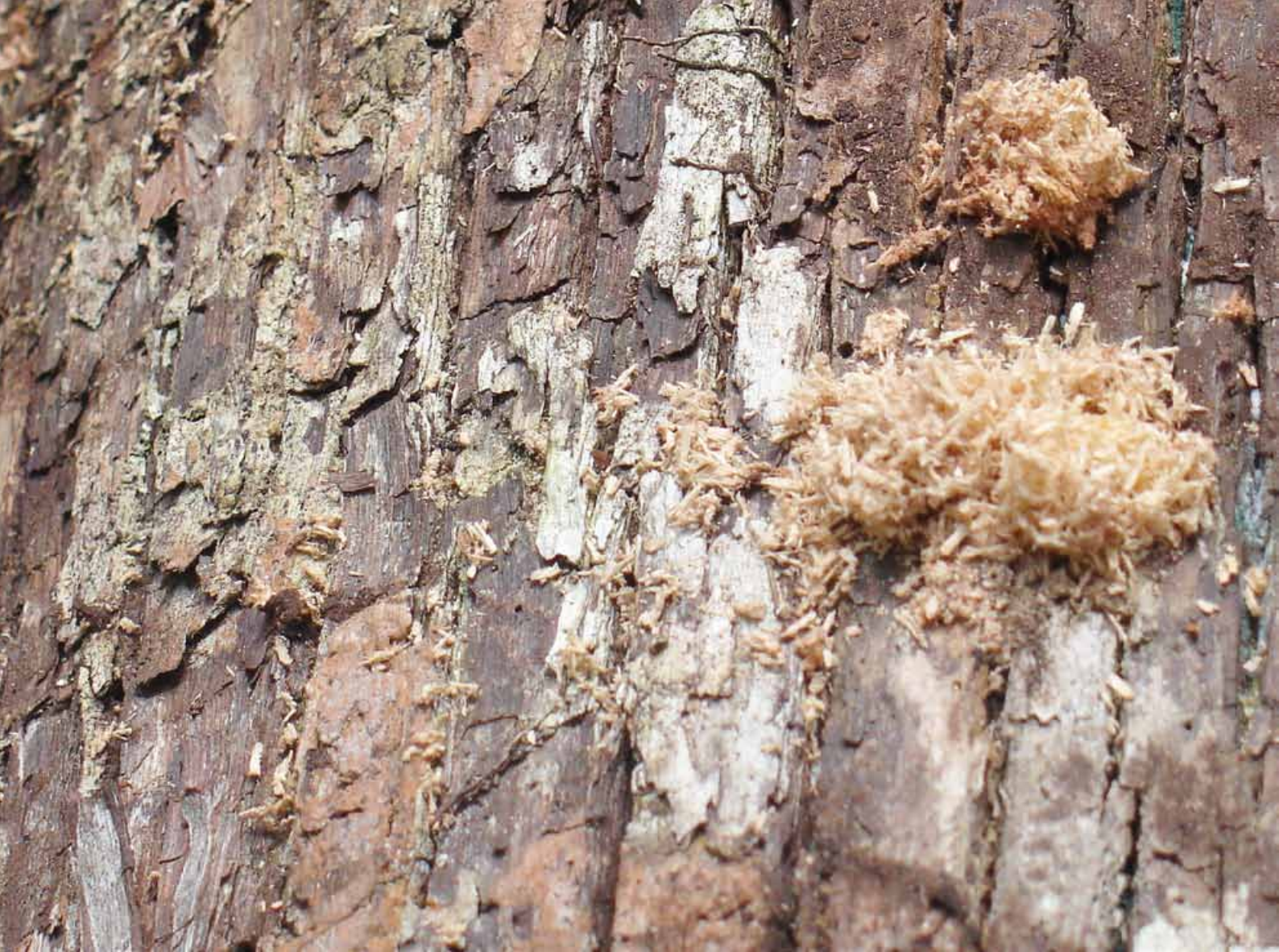
Figure 4.3 Powder-post beetle attack on G. bancanus log.
