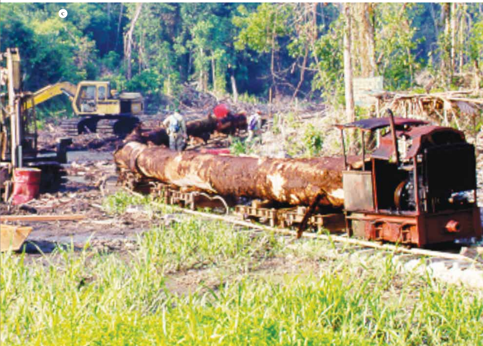
Figures 3.7 (a-c) Harvesting in the PSF of Selangor using modified traxcavator to extract the logs. Railway was used to transport the logs to the temporary log yard.
