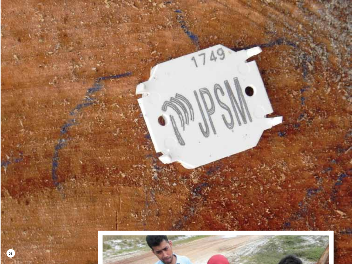
Figures 5.7 (a-b) Tag and equipment used for tagging and storing of G. bancanus information using the RFID technique.
