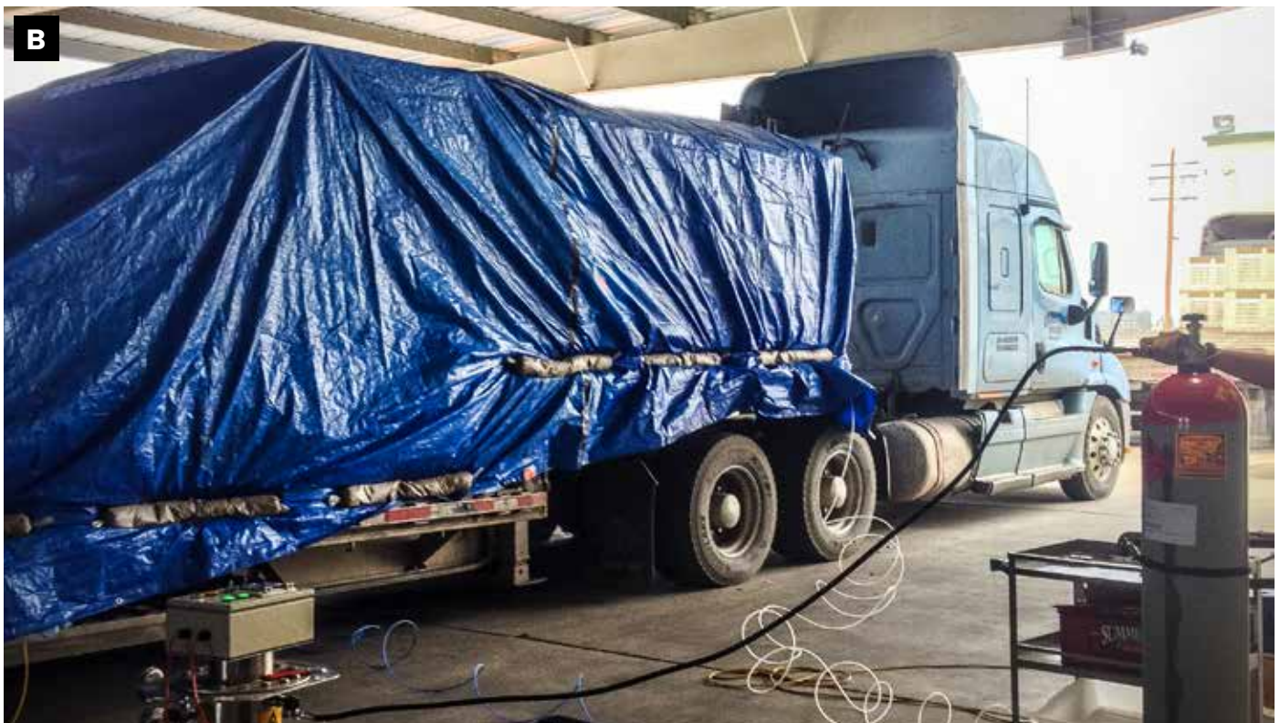
The application of eFUME requires a generator, which powers the volatizer that ensures cylinderized fumigant is expelled uniformly under the enclosure until the correct mass is applied, shown here during trials involving “curtain-side” (A) and “step deck” (B) trailers.
