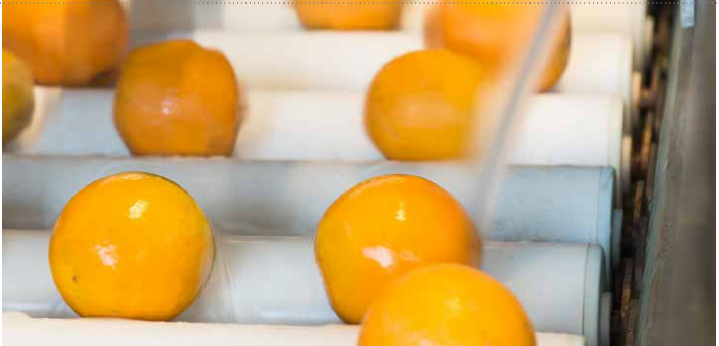
Figure 1. Post-harvest treatment of Valencia oranges using a recycling fungicide flooder application system containing an organic acid sanitizer to meet Food Safety Modernization Act (FSMA) regulations on sanitizing water systems in contact with food.
