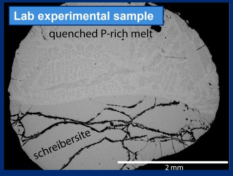
Lab experiments at APL produced samples that contained schreibersite, to replicate the chemistry found in the IIG meteorites
