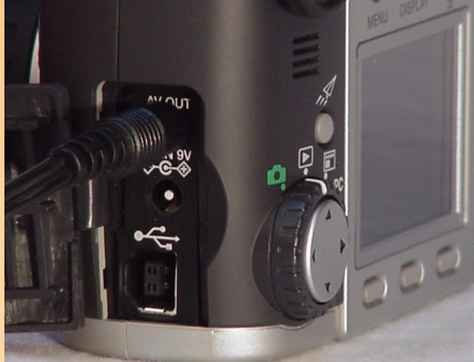
Figure 36: Connecting the Video Cable to the Camera
