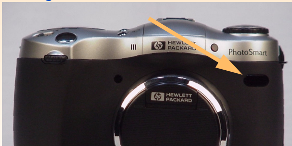
Figure 35: Infrared Window on the Camera
