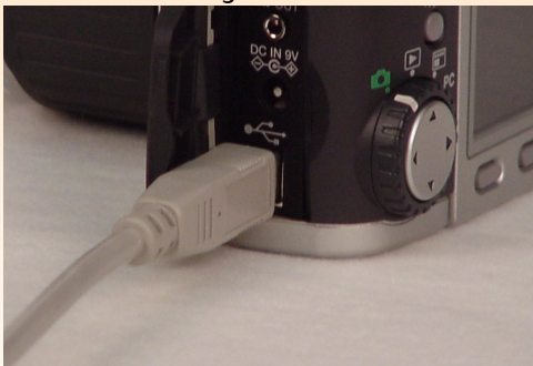
Figure 34: Connecting the USB Cable to the Camera
