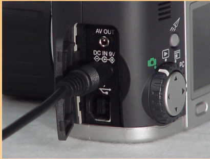
Figure 92: Connecting the HP AC Power Adapter's Cable to the Camera
