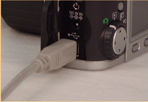
Figure 32: Connecting the USB Cable to the Camera
