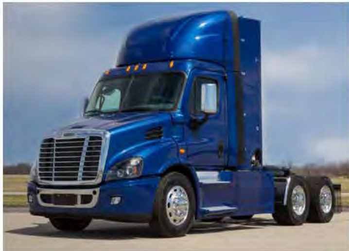
The Freightliner Cascadia is just one heavy-duty Class 8 tractor suitable for drayage that can be purchased today with a CWI 12-liter natural gas
