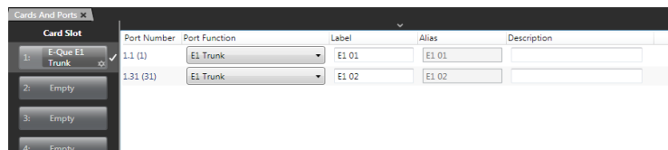
Figure 9-8 E1 Trunk Ports
