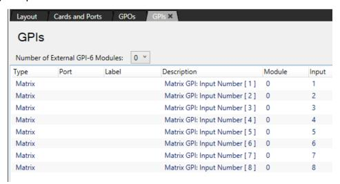
Figure 15-2 GPI-6 modules are added/removed from the GPI screen
