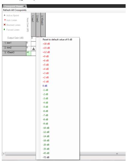
Figure 25-6 Input and Output Gain Settings
