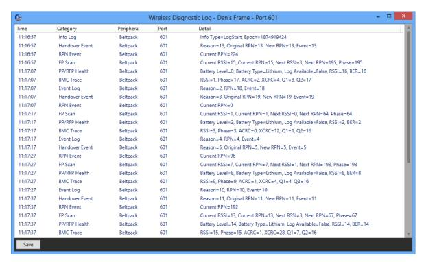
The static log window shows the same details as the live log window. When a log is saved, this is CSV format.
