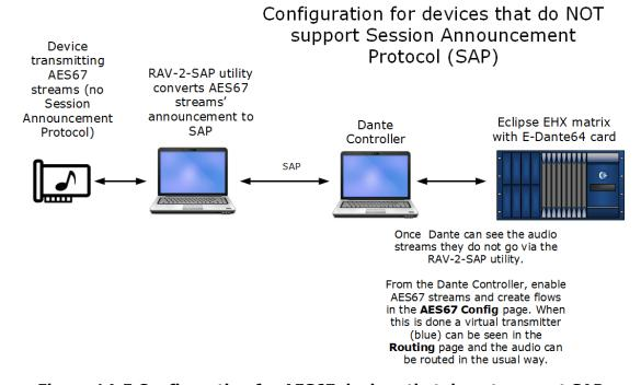
Figure 14-5 Configuration for AES67 devices that do not support SAP
