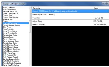
Figure 25-10 IP Address Setup Display
