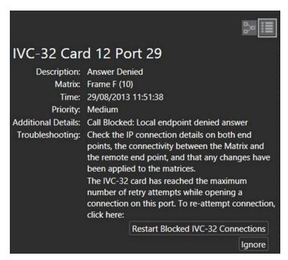
**Figure 23-9 Restart Blocked Connections**
