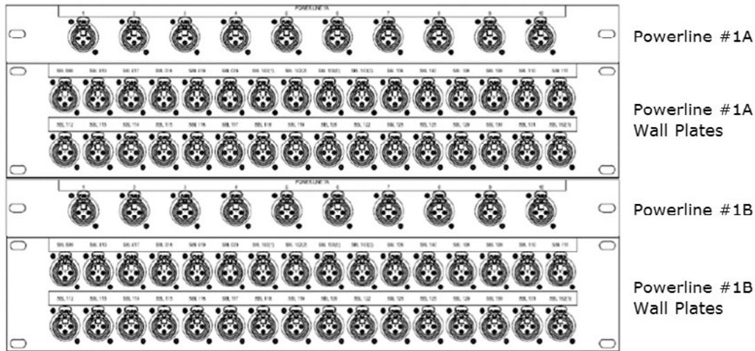
Figure 42: XLR Patch Panels
