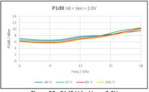
Figure 38: P1dB Vd = Ven = 2.0V
