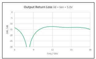
Figure 8: Output Return Loss Vd = Ven = 5.0V
