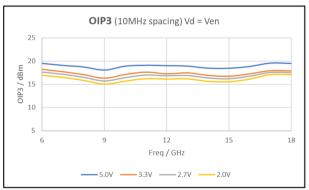
Figure 17: OIP3 (10MHz spacing) Vd = Ven
