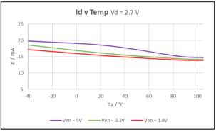
Figure 42: Id v Temp Vd = 2.7V
