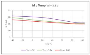
Figure 41: Id v Temp Vd = 3.3V
