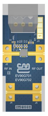
Figure 46: EV90G701 PCB Top Layer View
