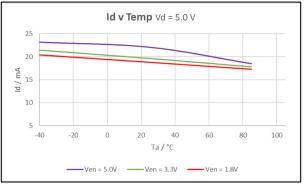
Figure 39: Id v Temp Vd = 5.0V
