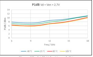
Figure 37: P1dB Vd = Ven = 2.7V
