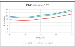
Figure 35: P1dB Vd = Ven = 5.0V
