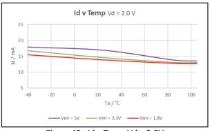
Figure 43: Id v Temp Vd = 2.0V
