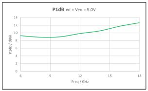
Figure 3: P1dB Vd = Ven = 5.0V
