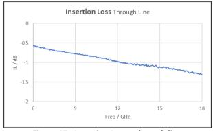
Figure 47: Insertion Loss – through line
