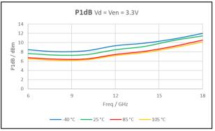
Figure 36: P1dB Vd = Ven = 3.3V
