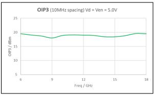
Figure 5: OIP3 (10MHz spacing) Vd = Ven = 5.0V
