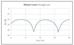
Figure 48: Return Loss – through line
