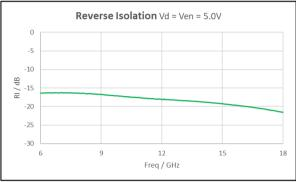
Figure 2: Reverse Isolation Vd = Ven = 5.0V
