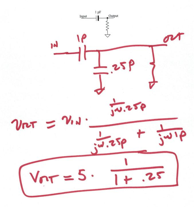
8. If the resistor value is 20k in the previous problem and an AC voltage is applied to the input estimate the frequency where the output AC voltage is half of the AC input voltage. Sketch the schematic of the equivalent circuit ensuring the bottom plate parasitic's location is clear. Please place a box around your numerical answer. As in all of the problems on this exam showing your work is important for getting full marks. (10 points)
