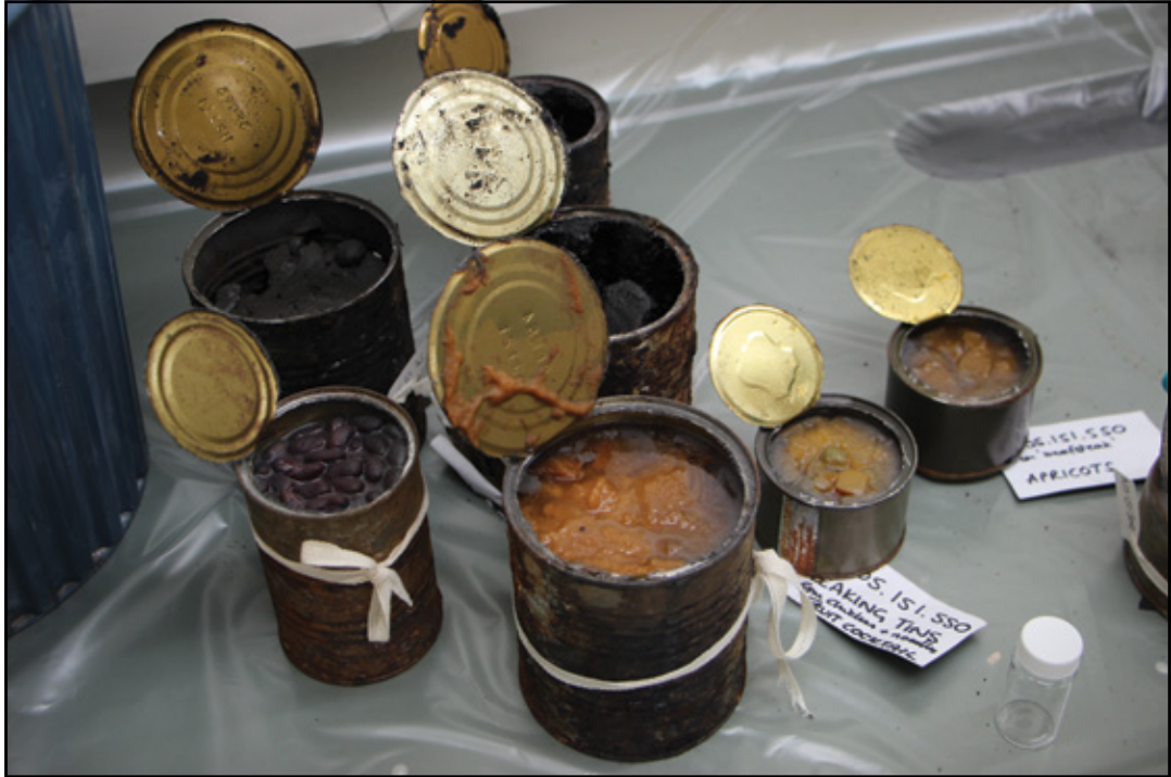
Figure 2. A selection of cans after opening with a rotary tool (L Yeats, 2014).
