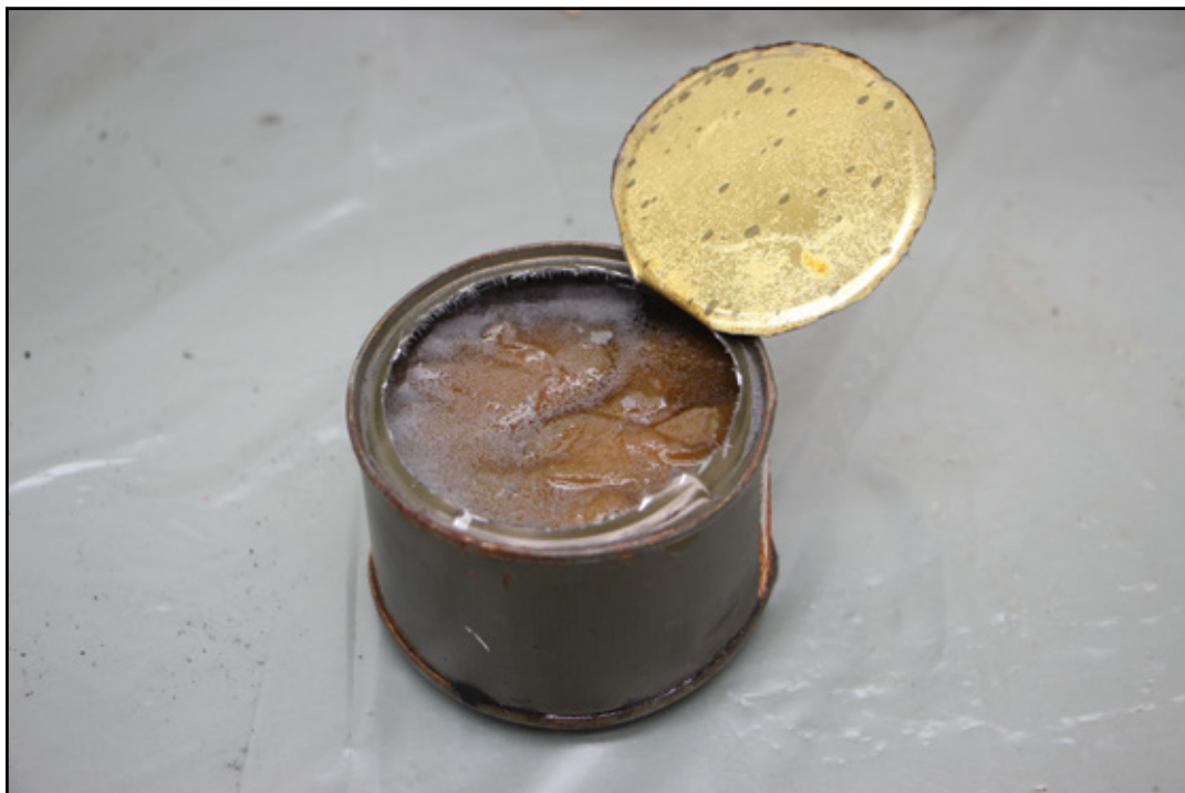
Figure 3. Open can showing fine metal filings (L Yeats, 2014).
