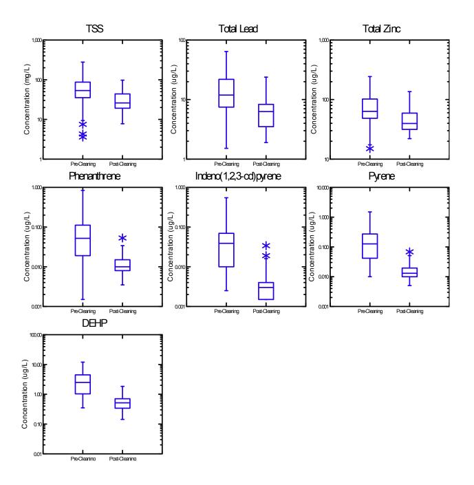
Figure 2-3.5 OF254 Storm Line Cleaning Comparison [Log Scale]
