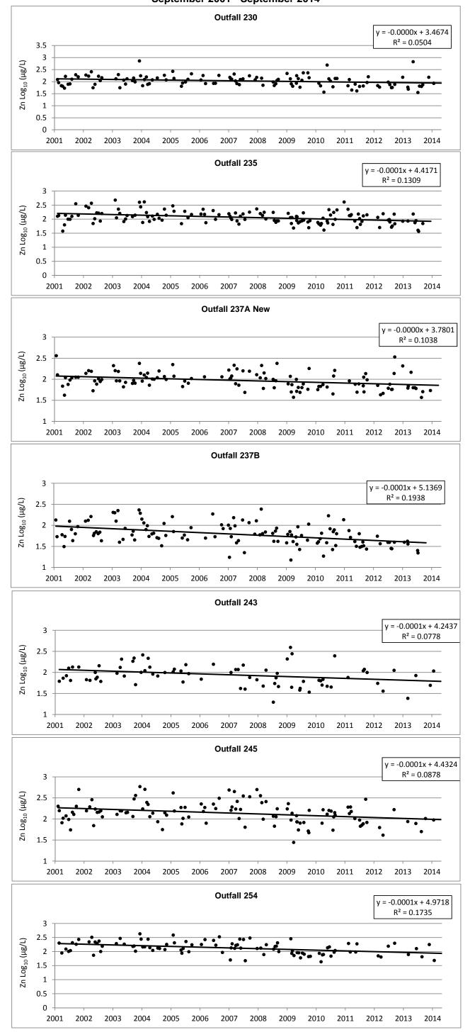
Figure 3-6.4 Linear Regression Analysis of Stormwater Time Trends Time Series for Phenanthrene September 2001 - September 2014
