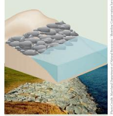
Lays over the slope of a shoreline. Protects slope from erosion and waves.
